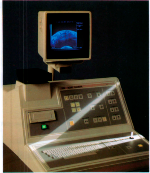
4. ALOKA Ultrasound thyroid scanner
