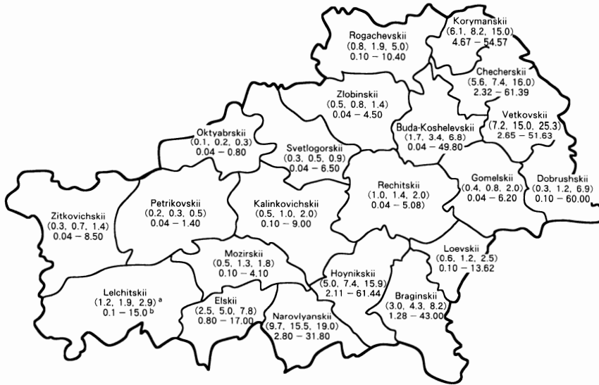
Figure 1. Cs-137 contamination levels ( \text{Ci}/\text{km}^2 ) in the rayons of Gomel oblast as measured in 1992.
